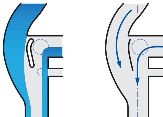
Bend to limit the speed of dropping water.
