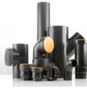
The Akatherm HDPE system has a full range which includes pipes, bends, junctions, reducers, traps and electrofusion couplers. Akatherm HDPE has high temperature and chemical resistance which makes it ideal for drainage in, apartments and commercial buildings through to industrial use. It is flexible and tough and can be installed underground and embedded in concrete.
