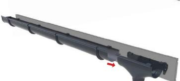
4. Once the solvent is set, insert the length of spouting into the brackets and slide into the expansion outlet. Align end of spouting to marking corresponding to the air temperature at the time of install.
