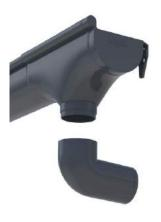
1. Connect the first bend to the expansion outlet. Note: For easy removal of the downpipe assembly for future cleaning and maintenance, screw rather than solvent weld the first bend to the outlet.
