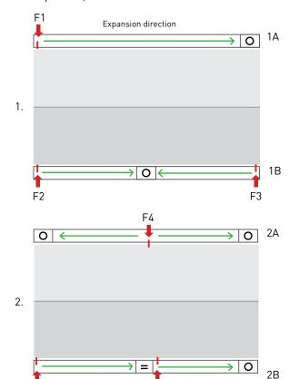
1A. For an expansion outlet positioned at one end of a spouting run, the expansion will be directed from the stop end to the expansion outlet. Fix at location F.
