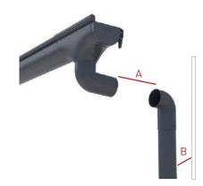
2. Calculate the offset length. When calculating the length of offset downpipe (A), include the length of sockets (30mm or 40mm each end depending on bends used and orientation) and take into account the gap (B) between the downpipe and the wall. (Refer Section 4.3 for downpipe clip dimensions).
