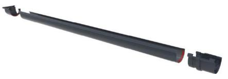
2. At ground level solvent weld the external angle and expansion joiner onto a spouting length. Let this assembly set for at least 10 minutes.
