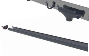
3. At ground level solvent weld the stop end onto a spouting length. Let this assembly set for at least 10 minutes.
