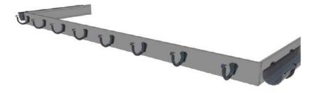
1. Fix the brackets to the fascia with correct spacing from high point to low point (refer to Section 2.1 page 8). Use the recommended fall to the outlet of 5mm per 10 metres.
