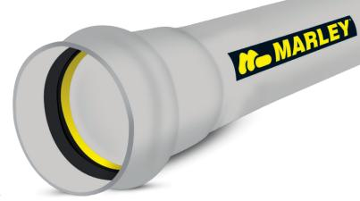
The system utilises advanced manufacturing technology to form the pipe socket and integrate the ring during the manufacturing process. This creates a secure and reliable seal with no further ring assembly required onsite.
