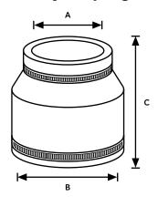
A and B Mean ID measurements are based on the resting internal bore of the coupling. All dimensions in mm. Ranges are based on a  $\pm$  5% allowance of stretch or contraction.
