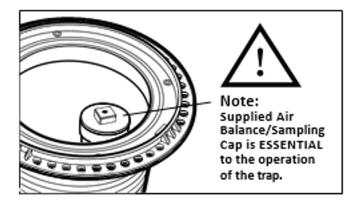
This assembly includes the Air Balance/Sampling Cap which is ESSENTIAL to the operation of the trap. When installing a Riser Extension (full or partial) it is necessary to extend and then relocate this important fitting.
