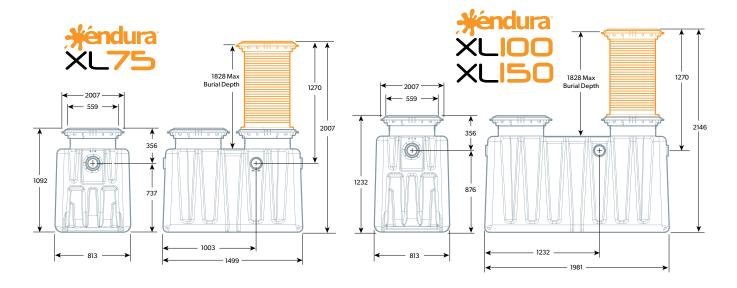
The maximum height above the top face of the body is 1,828mm. exceeding this limit may compromise the integrity of the body.
