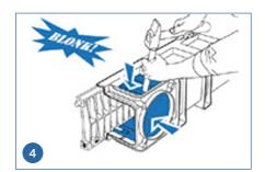
Hammer the desired outlet in and put into position the required outlet/stop end fitting.
