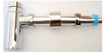
Measure extension tube from trap to wall connection, cut to required length and load bulkhead fitting, BSP nuts and sealing washers onto waste tube
