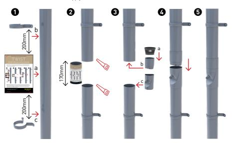
**Note:** Downpipe clip fixings not included - purchase separately to suit your cladding type. Twist should be installed higher than the inlet point to a small tank. Twist should not be installed on metal or rectangular downpipe or on downpipe larger than 80mm OD. If installing Twist on 65mm uPVC downpipe extra adaptors are required.
