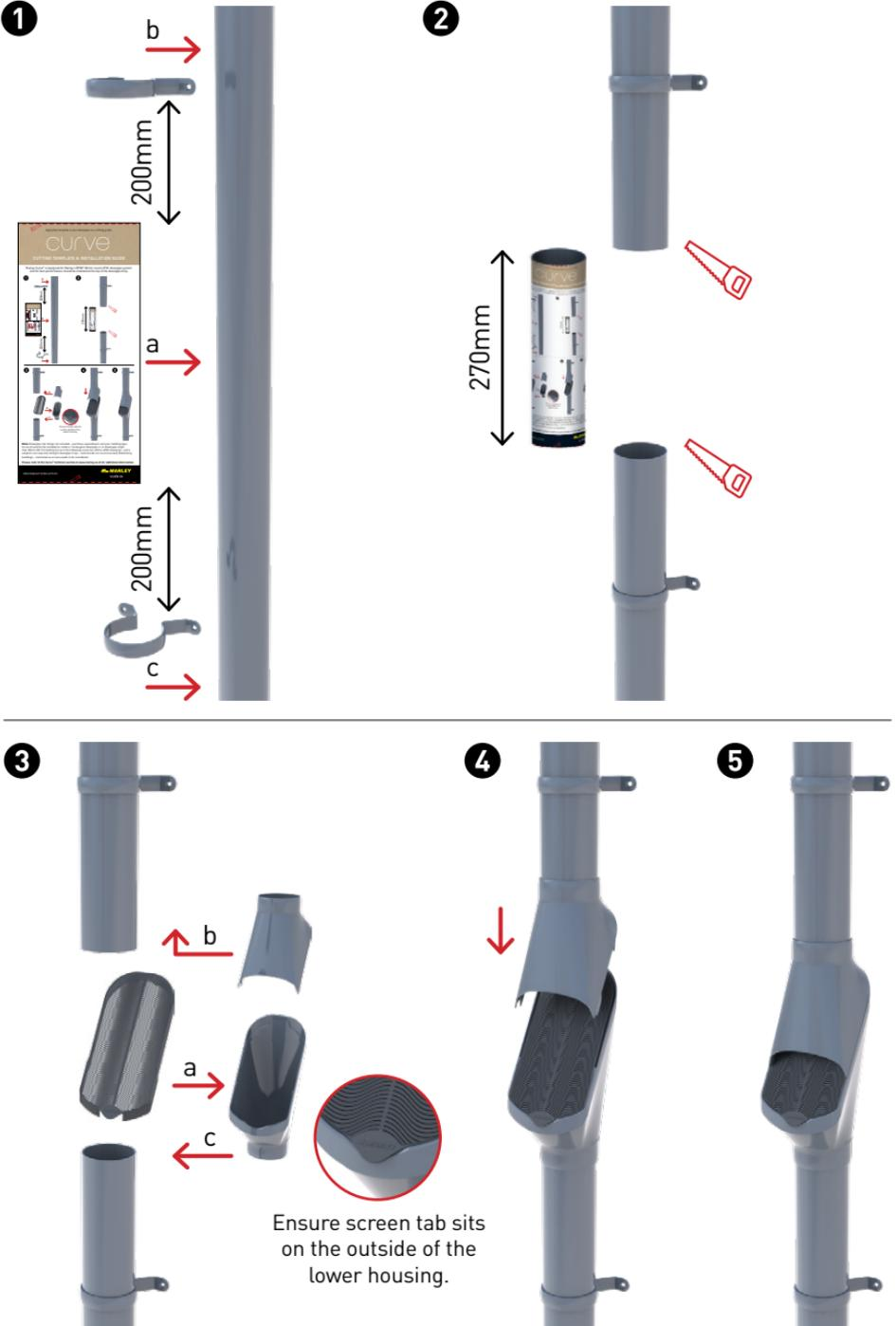
**Note:** Downpipe clip fixings not included - purchase separately to suit your cladding type. Curve should not be installed on metal or rectangular downpipe or on downpipe larger than 80mm OD. If installing Curve in the following scenarios: 65mm uPVC downpipe - extra adaptors are required; Straight downpipe drops - extra bends are recommended; Multistorey buildings - maintenance access needs to be considered.
